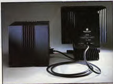
Photo 2: The monitor I/O ports, left to right: stereo earphone jack, left and right stereo channels, umbilical connection, keyboard connector, microphone jack.
