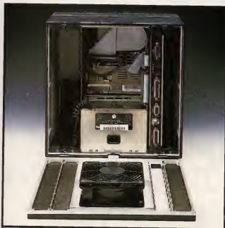
Photo 4: The inside of the cube. At top center is a bay for an additional full-height peripheral; at center is the magneto-optical drive. The power supply is at the bottom. To the right of center is the main CPU board.
